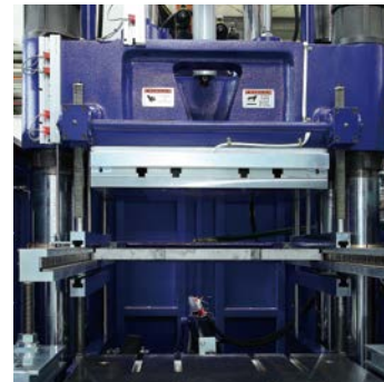
Top/ Bottom Hydraulic Mechanical Ejectors, Synchronized Mechanism 上/下吊模裝置、同步機構
